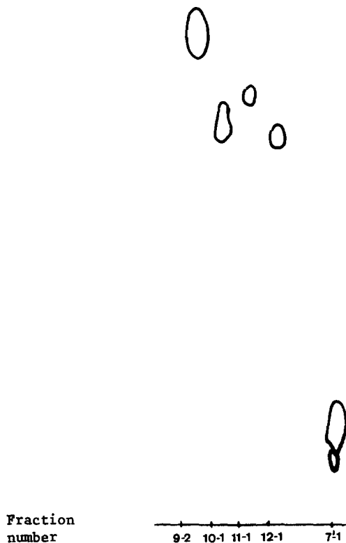
Fig. 9. Analytical OPLC of apricot glycosidically bound fractions obtained after preparative OPLC on 0.2-mm silica gel (Kieselgel 60). Eluent, ethyl acetate- tert. -amyl alcohol-acetic acid-water (18:1:1:1, v/v) at a flow-rate of 0.75 ml min -1 . Nediac reagent was used for detection.
